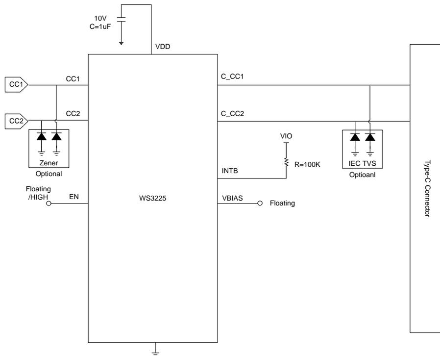
**Note:** For the WS3225C, If TVS are all used in the C\_CCx pins, the VBIAS pin can be floating without 100nF capacitor.
