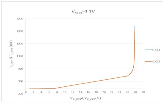
$V_{C\_CC1} \& V_{C\_CC2}$  vs  $I_{C\_CC1} \& I_{C\_CC2}$  ( $V_{DD} = 3.3V$ )
