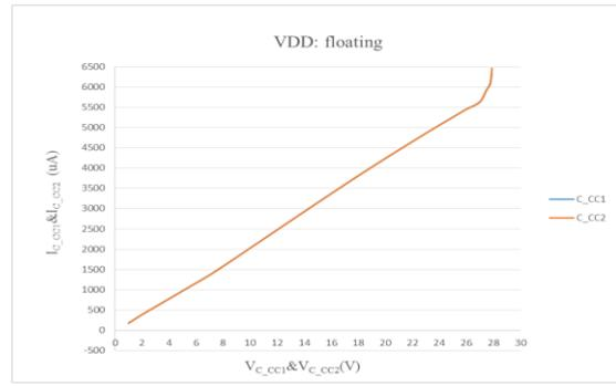
$V_{C\_CC1} \& V_{C\_CC2}$  vs  $I_{C\_CC1} \& I_{C\_CC2}$  ( $V_{DD} : \text{floating}$ )
