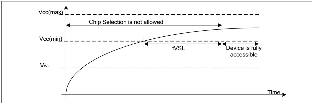
Table 24 Power-Up Timing and Write Inhibit Threshold
