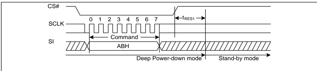
**Figure 57 Release Power-Down/Read Device ID Sequence Diagram**
