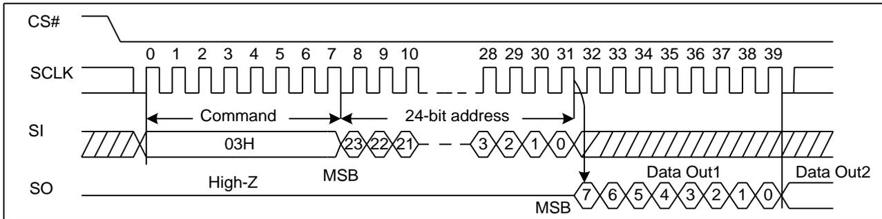
**Figure 10 Read Data Bytes Sequence Diagram (ADS=1)**
