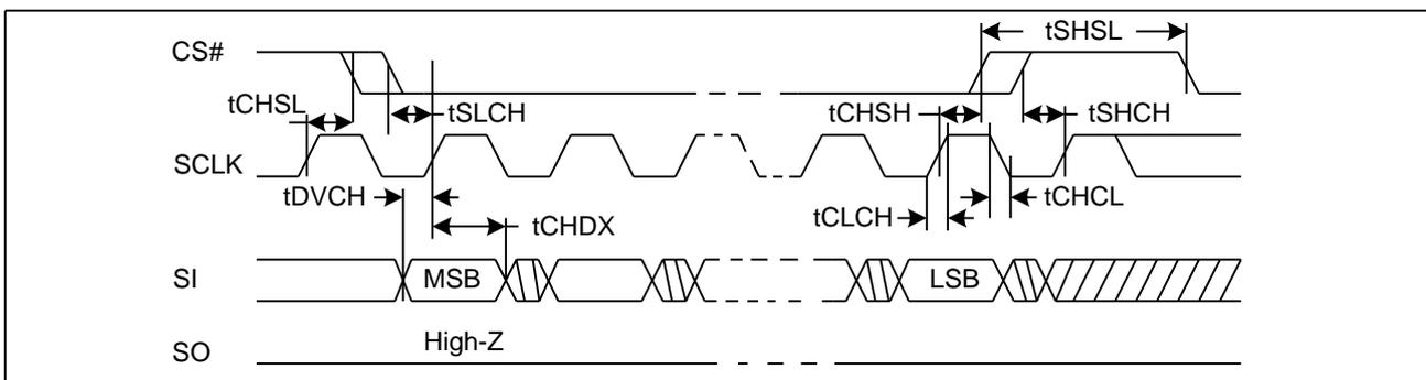
**Figure 75 Output Timing**
