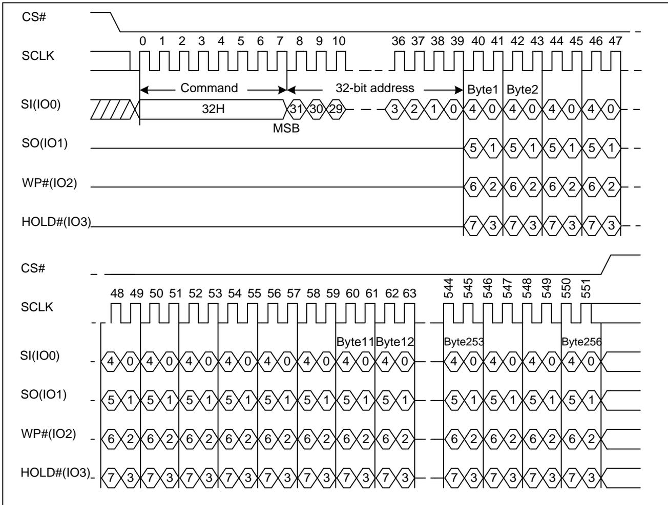
Figure 39 Quad Page Program with 4-Byte Address Sequence Diagram (ADS=0 or ADS=1)
