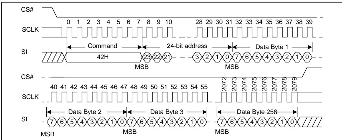
Figure 65 Program Security Registers command Sequence Diagram (ADS=1)
