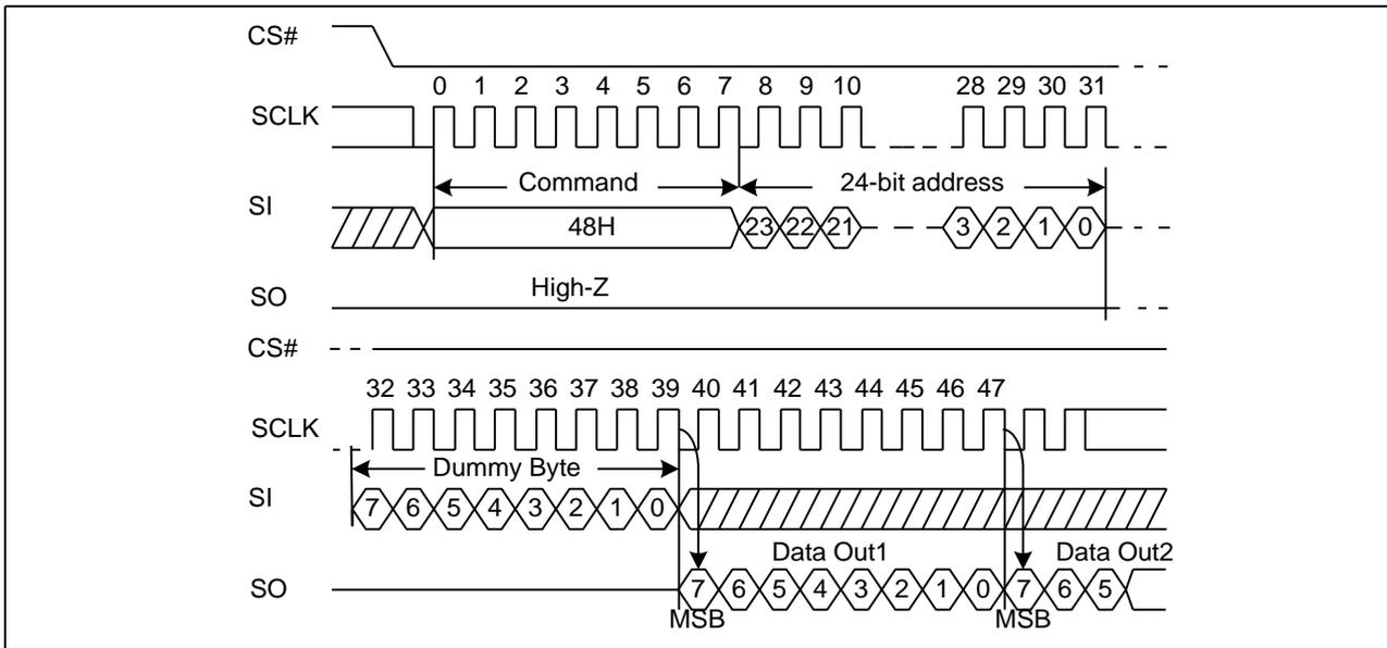
**Figure 67 Read Security Registers command Sequence Diagram (ADS=1)**
