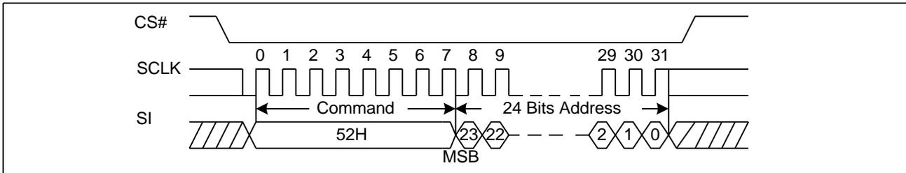
**Figure 44 32KB Block Erase Sequence Diagram (ADS=1)**
