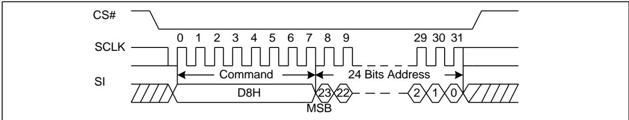
**Figure 47 64KB Block Erase Sequence Diagram (ADS=1)**
