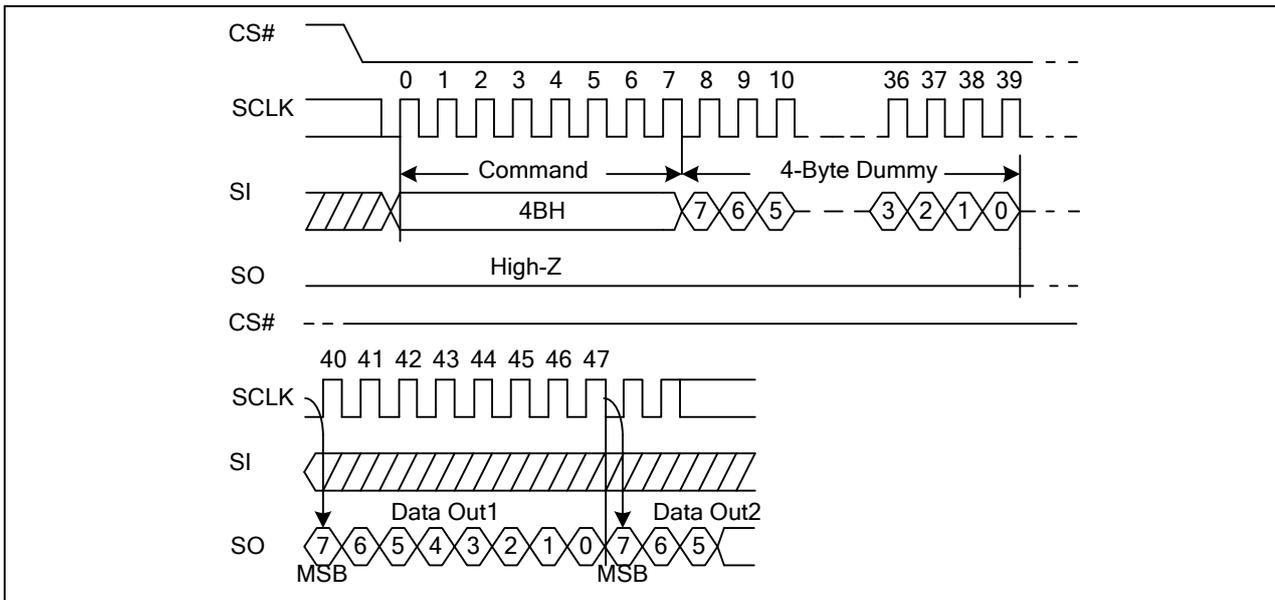
Figure 52 Read Unique ID Sequence Diagram (ADS=1)
