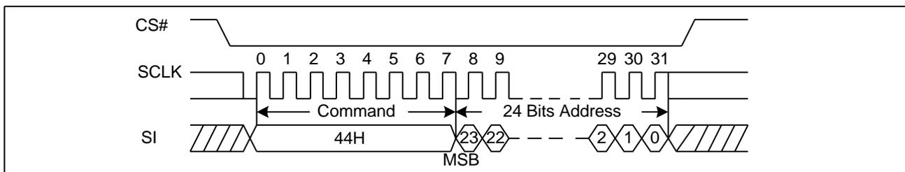
**Figure 63 Erase Security Registers command Sequence Diagram (ADS=1)**
